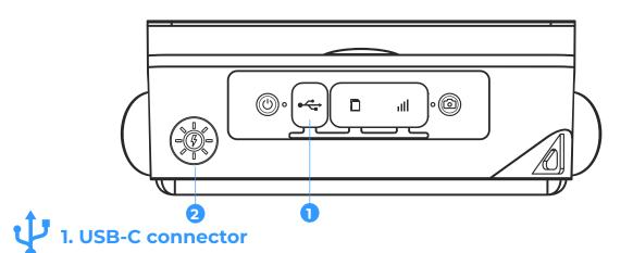
This connector is used notably for the Tikee's first charge. Caution : when plugged in, this connector is not waterproof.
