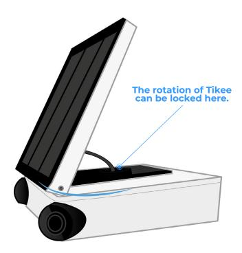
Start by orientating the solar panel to the south if you are in the northern hemisphere, or north if you are in the southern hemisphere. You can use a compass, a watch with a compass function or a mobile application on your smartphone
