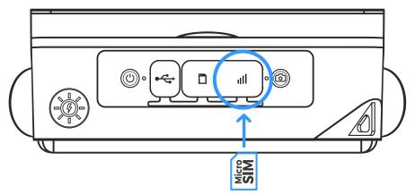
Inserting the SIM card: Metal contacts of the chip downwards, angle left to the bottom - see above.
